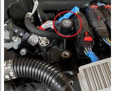
Connect short hose with 45 degree fitting onto intake manifold fitting, connect the longer hose with the 90 degree fitting to the PCV value on the value cover. **TIP**: The quick connections are all adjustable in the end of the hoses, if the fitting isn't at an optimum angle, twist the fitting until it is. The hoses can also twist on the J&L Oil separator connections for adjustment.
